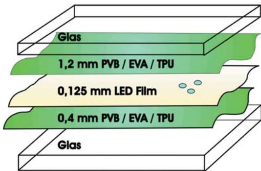
**Fig. 1 - Typical specification of laminated glass using LED embedded films**
